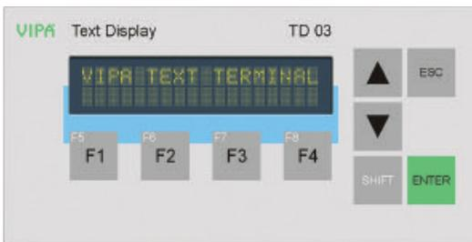
S7-300/400® PLCs and VIPA series 100/200/300V PLC's. The configuration is done with the VIPA TD-Wizard. The generated parameters and data blocks are directly loaded in the PLC. The TD itself contains no project data.
