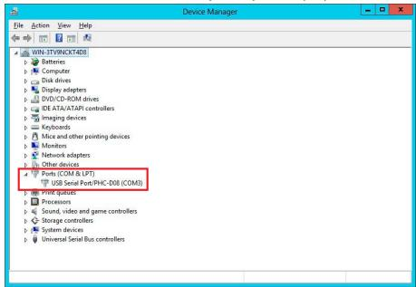
\* Make sure the connected product model is displayed after the "USB Serial Port/" prefix.
