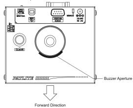
•When installing this product, pay attention to the mounting direction since the buzzer sound level is at it's maximum towards the front.
