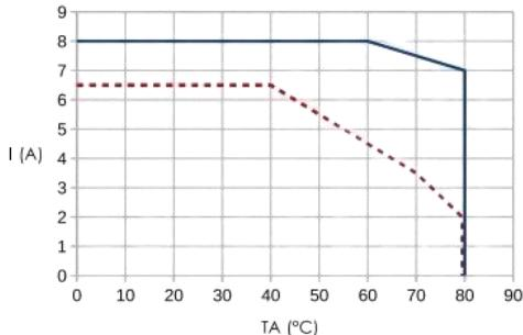
— SSR Installato singolarmente / Stand alone installed SSR
