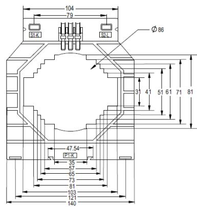
**GOGAFACE SPCT Stromwandler / current transformer**
