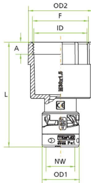
**GOGACON SF NÄHERUNGSSCHALTER-ADAPTER / proximity switch adapter**
